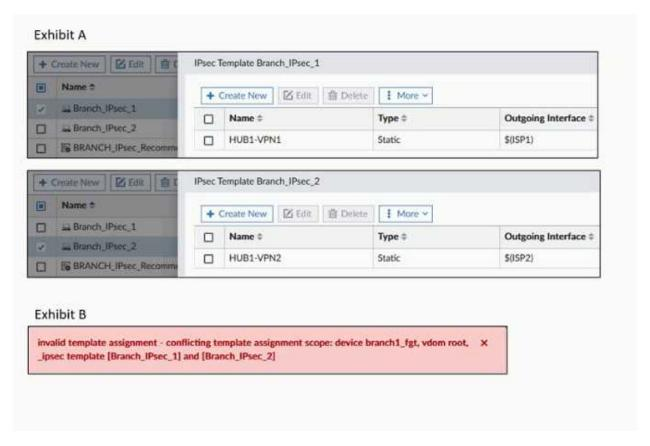
Exhibit A shows two IPsec templates to define Branch\_IPsec\_1 and Branch\_IPsec\_2. Each template defines a VPN tunnel.
